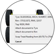
Right-click on any of the vehicle's positions to view fitment information. This is good practice to ensure you are removing and fitting the correct tyre/rim. You also have the opportunity to swap tread readings if the tyre has been turned on its rim.
